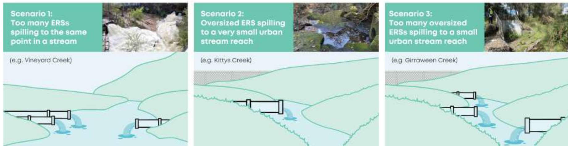
Figure 8-7: Conceptual model raised from investigating adverse ecological effects in receiving waters from WWOs
