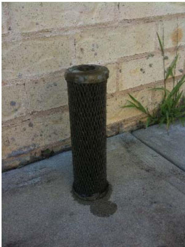
Figure 40: Clogged water filter limiting flow from rainwater tank pump in highest energy intensity household
