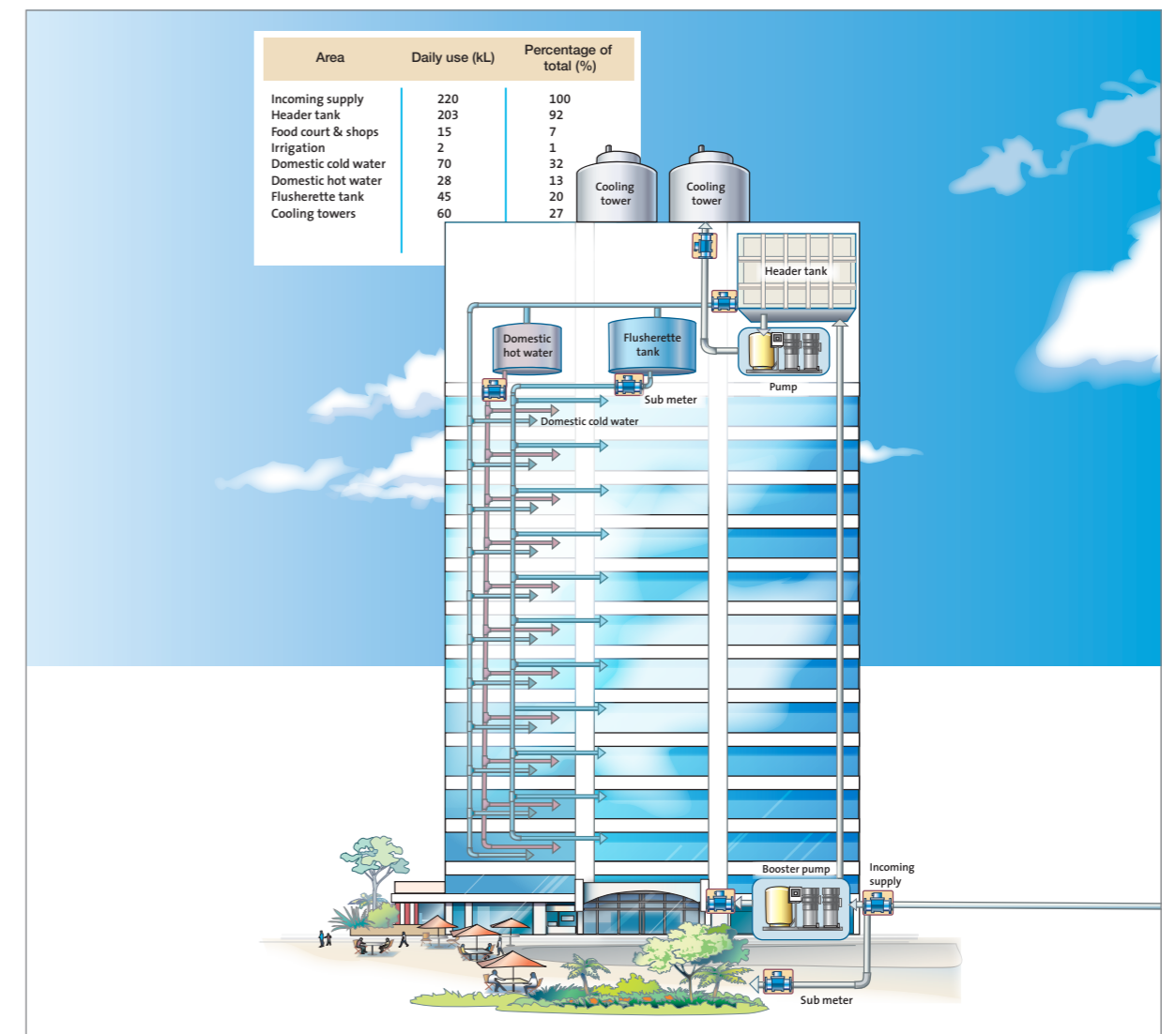
Figure 13 – A typical hydraulic system for a commercial office building shows suggested locations for sub meters. Once installed, these sub meters will allow an accurate water balance to be developed
