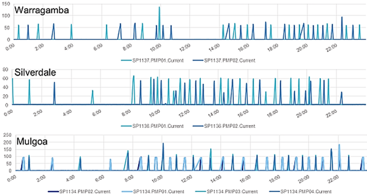
Figure 3-10 Example of network impact of influent flow
