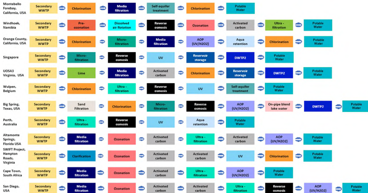
Figure 4-34 Configuration examples for direct and indirect potable re-use 1
