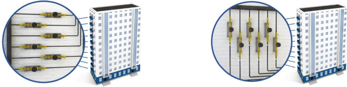
Figure 12. You can install meters either horizontally or vertically.
