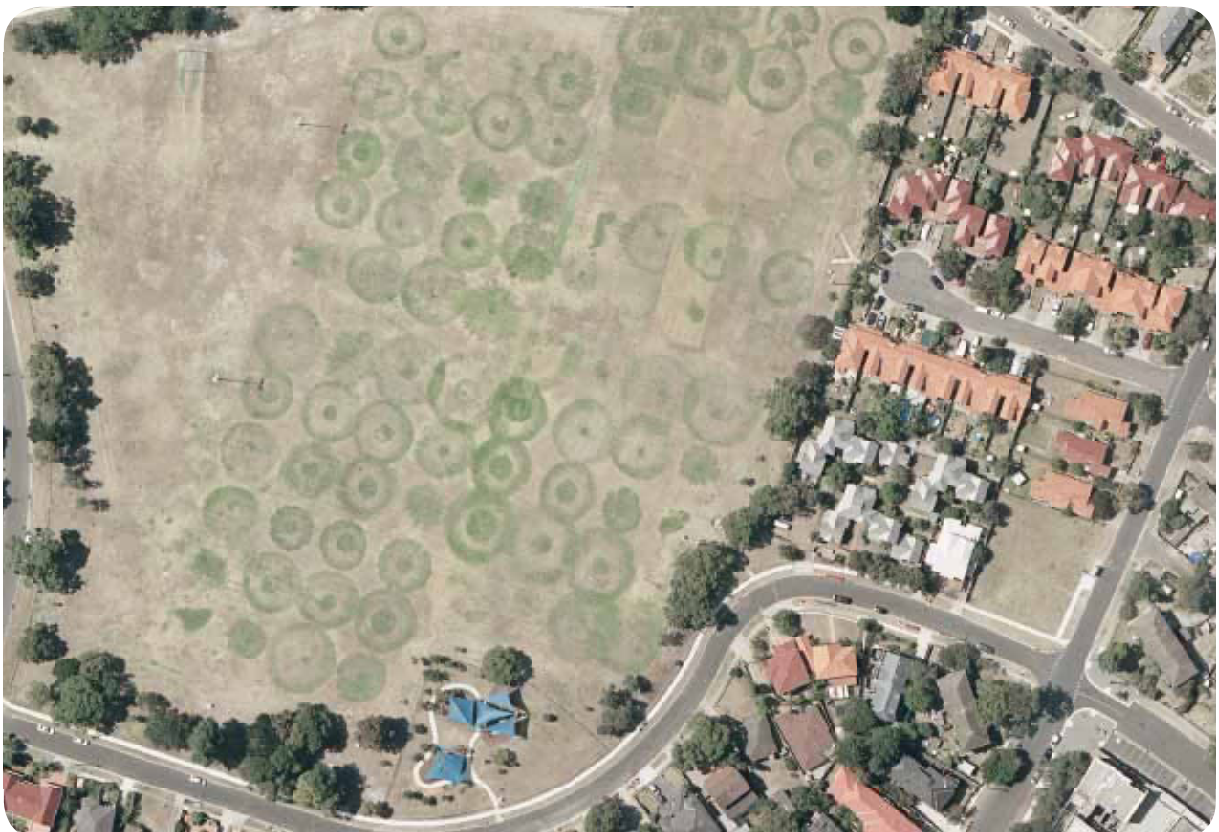
Figure 24 – The effect of poor DU on turf performance (ie green rings)
