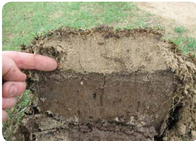
Figure 9 – Soil layering caused by top-dressing with too sandy a soil mix 24
